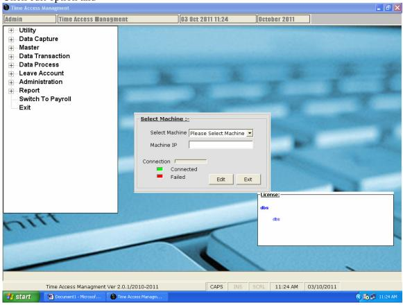
Machine id 1, machine name DTK 401 IP address 192.168.0.224/192.168.1.224 any ip according to your network port no is **5005**
